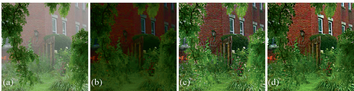
Figure 3 Visual comparison of the dehazing results of these methods for a heavy foggy color image. These methods are [20,21] and the proposed algorithm using image filtering approach. (a) Original image, (b) [20], (c) [21], (d) the proposed algorithm.
